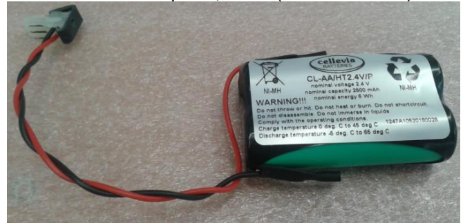
Akupack 2x 1200mAh, conductors 0,25mm 2 , l = 160mm, connector Panduit 2poles, cover (ME374000.368)
